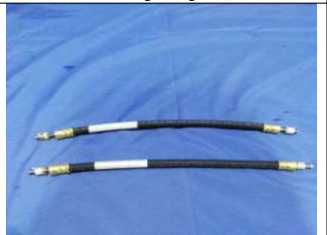
Photo 6 Bursting strength after test
