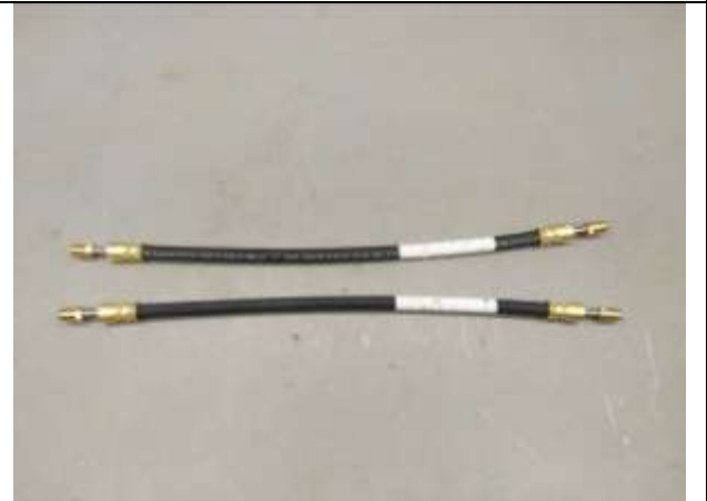
Photo 4 Bursting strength before test
